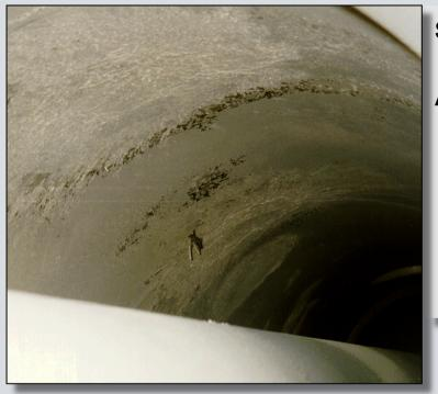
View inside the GIL: Test Conditions: 63 kA, 500ms Scenario: - fault detection by protection system - line drop-off and arc extinguishing Auto Reclosure:
